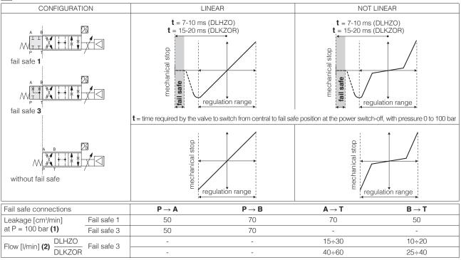
(1) Referred to spool in fail safe position and 50°C oil temperature (2) Referred to spool in fail safe position at  $\Delta p = 35$  bar per edge
